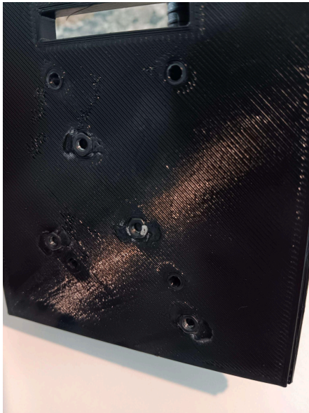
Figure 6.1.6 - Pressed M3 nuts
