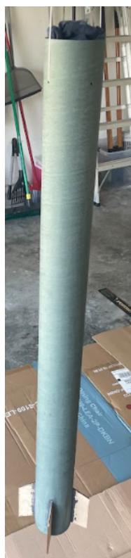
Figure 3.3.1 - Unpainted Rocket Chassis using Blue Tube Material.
