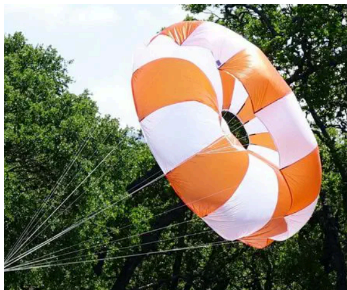
Figure 3.5.2 - 36" inflated parachute with exposed apex vent
