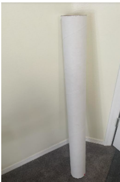
Figure 6.4.2 - Cardboard Test tube used to drop test eggs
