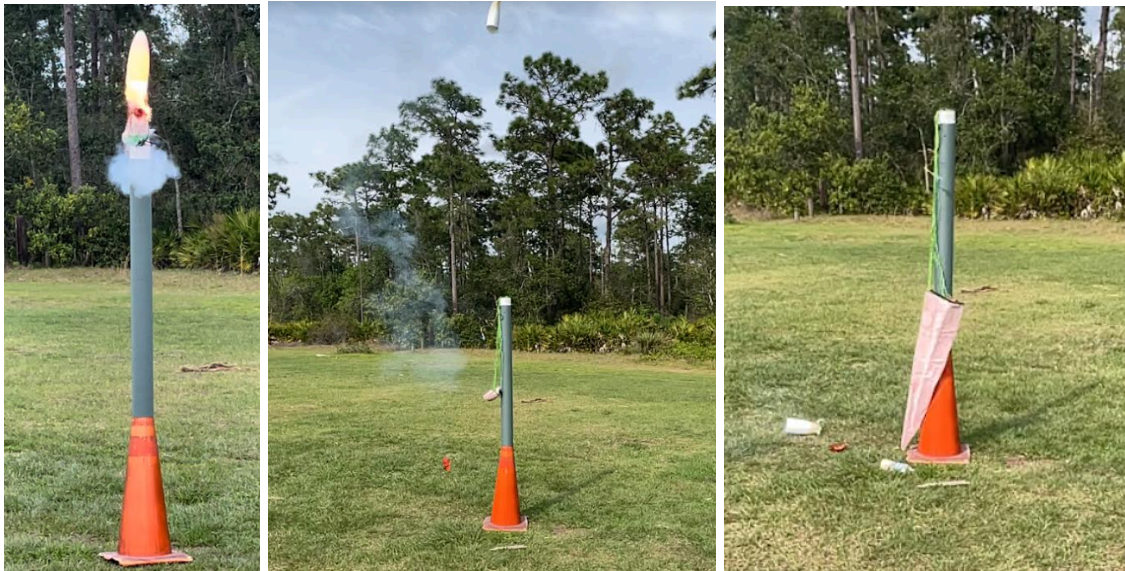
Figure 3.5.3 - Nose cone ejection and parachute deployment testing.
