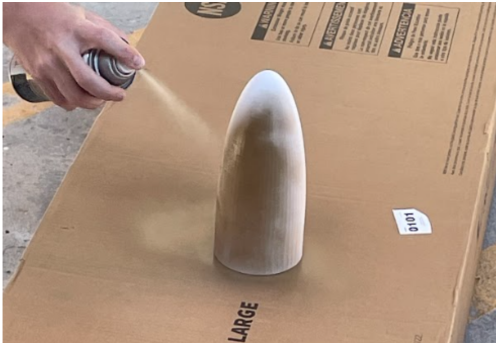
Figure 3.4.1 Parabolic nose cone made from poly-carbonate
