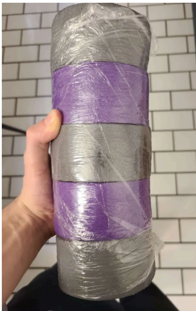
Figure 3.6.4 - Egg carrying pucks stacked in series and wrapped in cellophane.
