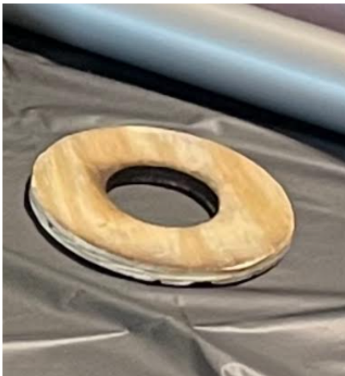
Figure 3.7.4 - 1/4" pine plywood centering rings.
