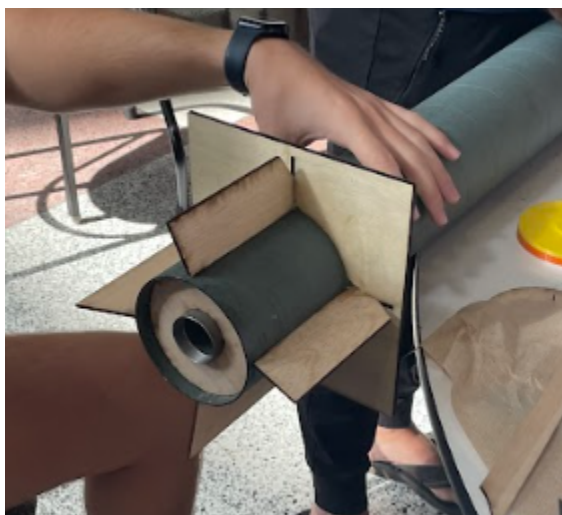
Figure 3.3.2 - Trapezoidal fin design with fin guard
