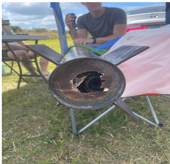
Figure 10.5 Centering Ring Failure
